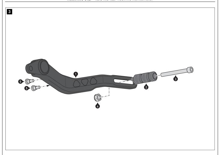
Screw the parts shown together. **A WARNING: Use liquid thread locker (cradle suspension (5))**Tighten the cradle suspension (5) as specified in the mounting instructions. Do not tighten the screw (3) yet.
