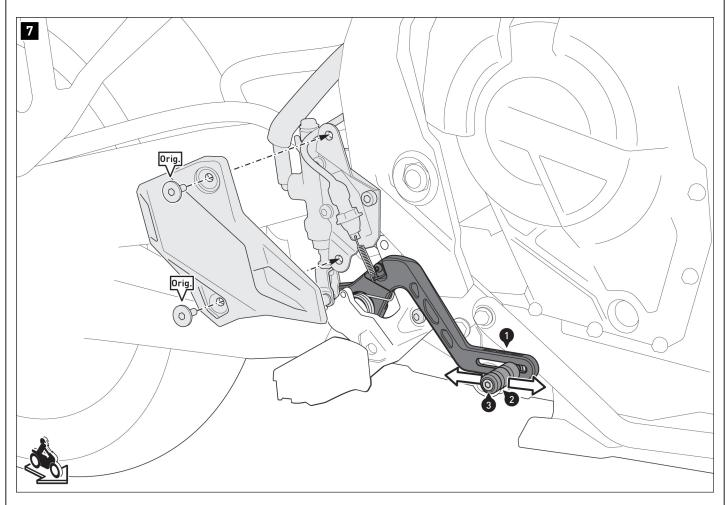
Adjust the pedal (2) according to your driving habits. Then tighten the screw (3) as specified in the mounting instructions.
