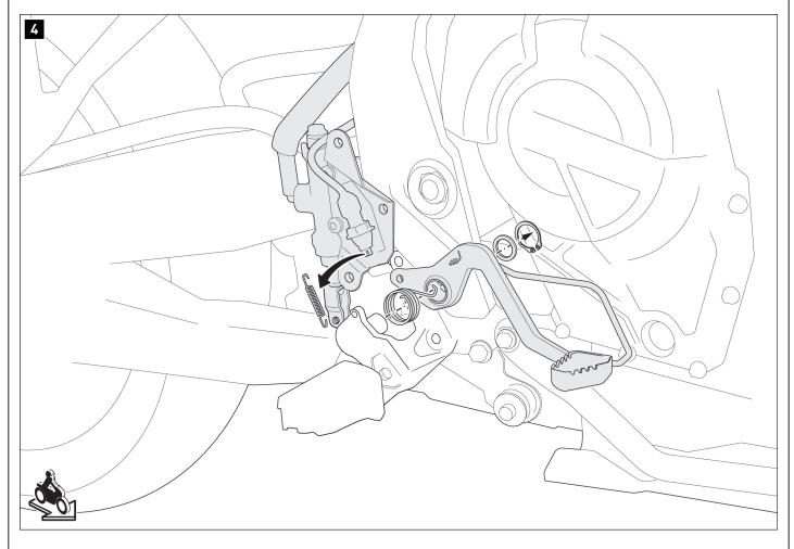
Loosen the springs and locking ring, and remove the original gear lever from the vehicle.
