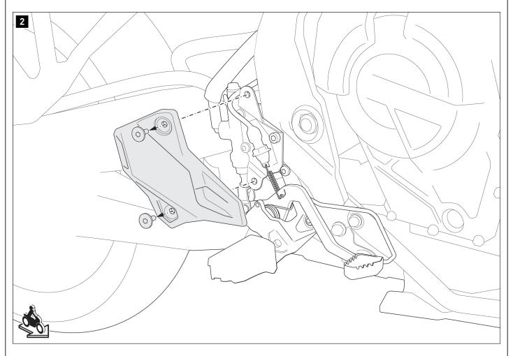
Loosen the screws, and remove the heel guard from the vehicle.
