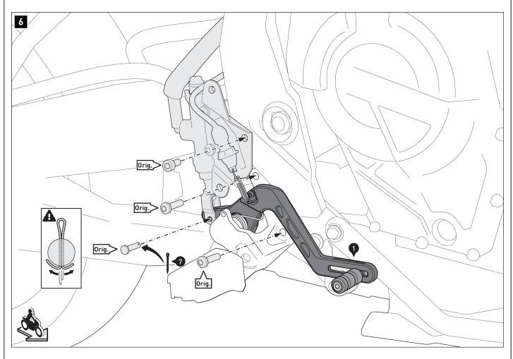
Connect the brake pedal (1) to the brake master cylinder. Use the original parts (Orig.) and the cotter pin (7).
