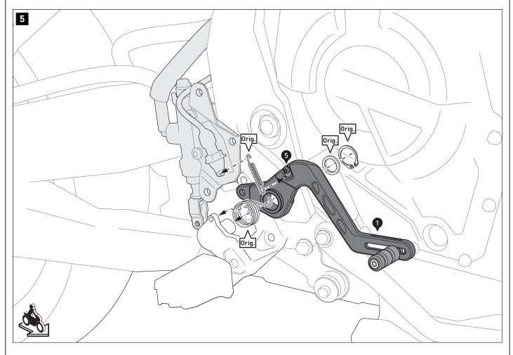
Attach the brake pedal (1) to the footrest mount using the original parts (Orig.).
