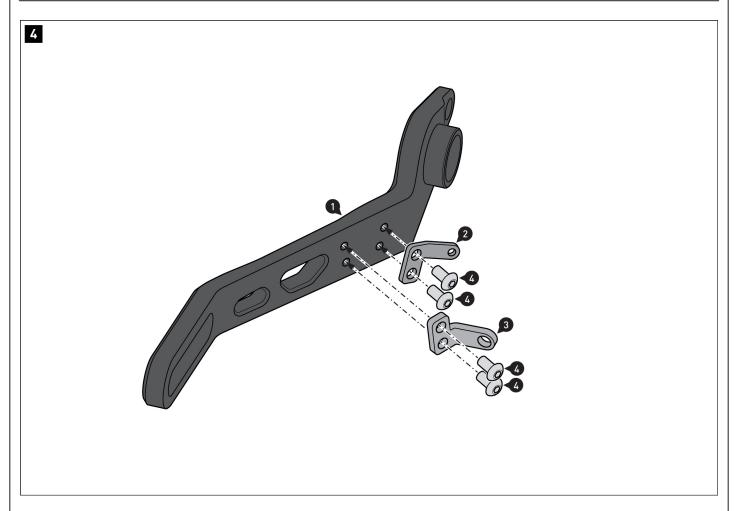
Screw the parts shown together. **A** WARNING: use liquid thread locker!
