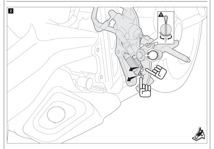
Loosen the cotter pin from the master cylinder push rod. Unhook the indicated springs. Remove the snap ring.
