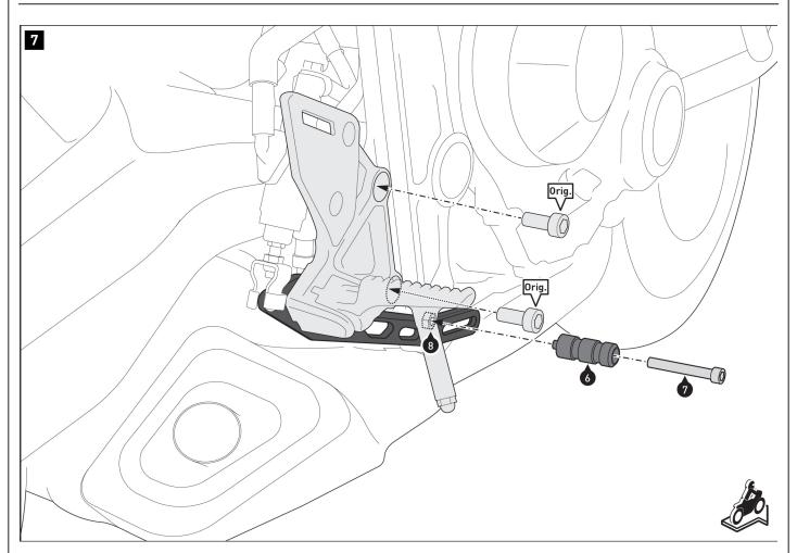
Screw the pedal (6) onto the brake pedal. Do not tighten the screw (7) yet.
