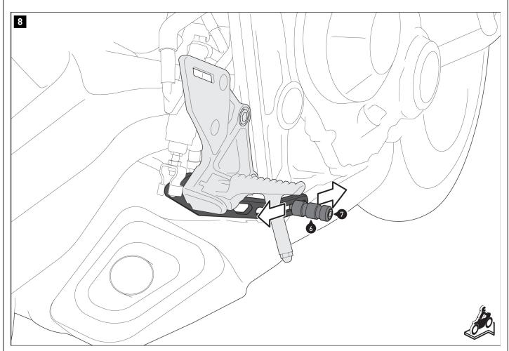
Adjust the pedal (6) according to your personal preference. Then tighten the screw (7) as specified in the mounting instructions.
