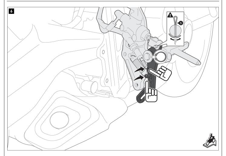
Hang the springs in the indicated position. Mount the original pressure rod (Orig.) using the **new** cotter pin (5). Attach the original snap ring.
