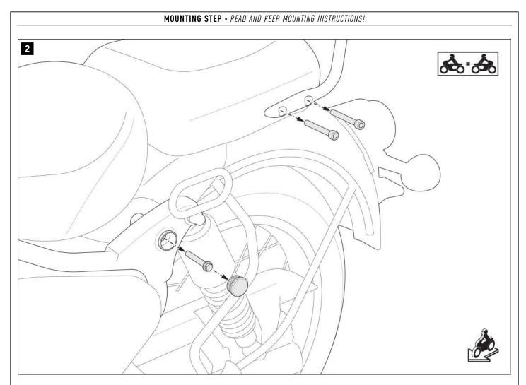
Remove the indicated cover cap and screws from the vehicle.
