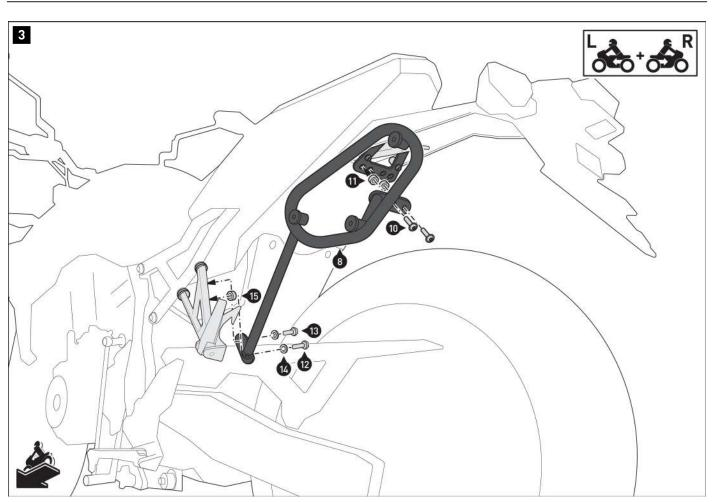
▲ NOTE: The spacers (11) are not required if mounting the SW-MOTECH rack at the same time.
