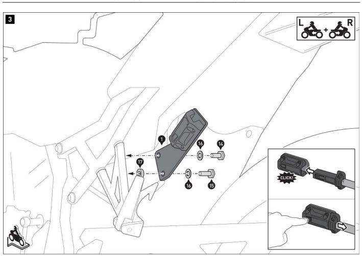
Screw mounting brackets [1] and [2] onto the passenger footrest mounts. **A WARNING: Use a liquid threadlocker!** Tighten the screws according to the manufacturer's instructions.
