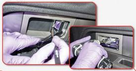
USE A FLATHEAD SCREWDRIVER OR PANEL TOOL TO POP OFF REMOVE THIS 8MM SCREW. THIS TRIM PIECE.
