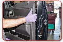
YOU CAN NOW LIFT UP ON THE DOOR PANEL. THERE ARE STILL PARTS ATTACHED TO THE DOOR ITSELF. DO NOT REMOVE THE PANEL COMPLETELY.
