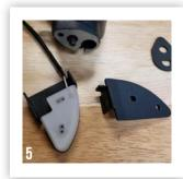
(6) Install new turn signal by screwing to top sheet metal
