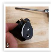
Take rubber mount, wrap back around fork, reinstall retaining bolt, route connectors back to OEM connector and plug back in
