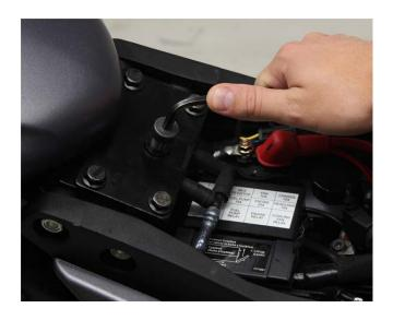
2. Remove the plug from the fender, revealing an 8mm threaded hole.
