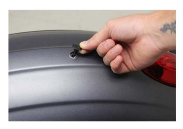
3. Engage the Mustang seat's front bracket with the shoulder screw and lower the seat to the fender.
