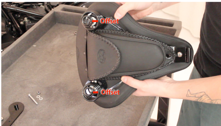
Make sure the offset (wider, more open) side of the spring is facing towards the front of the seat when tightening in place.
