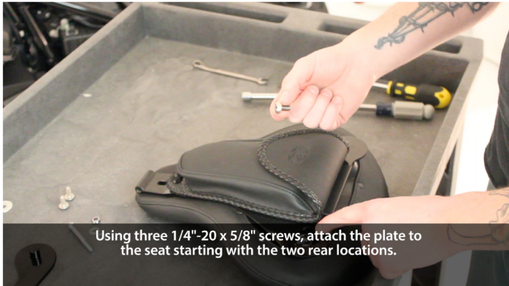
On the underside of your solo seat there are three 1/4"-20 mounting locations.
