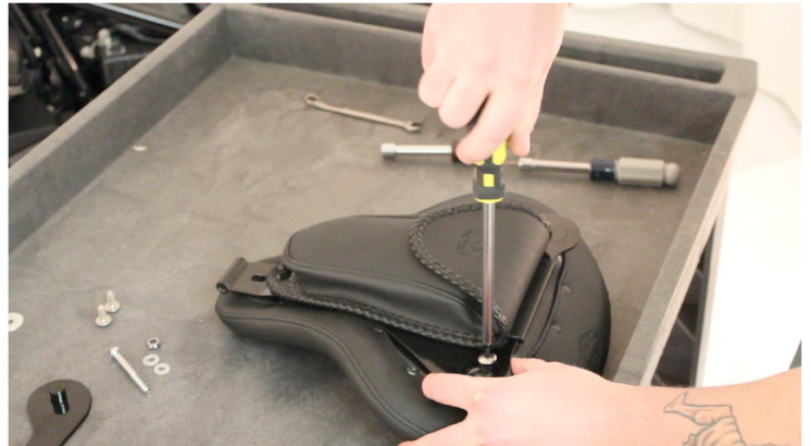
Line up the three holes in the mounting plate with the holes on your seat.
