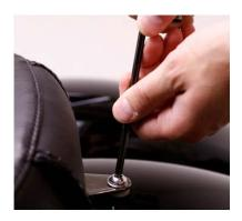
4. Push the seat fully forward until the rear bracket aligns with the fender mount and, using a 5mm Allen wrench, secure to the fender with the stock rear screw, grommet and washer. Indian recommends torquing this bolt to 8 ft-lbs (96 in-lbs, 10.8 Nm).
