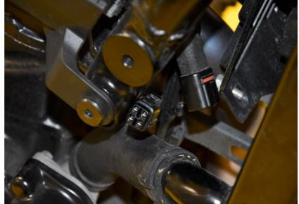
Plug the OSE connector into the wiring harness connector.
