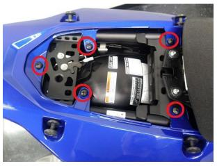
Remove the 6 silver 8mm head screws from the Left and Right under side of the tail section
