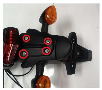
14) Cut all cable ties retaining the wires to the fender assembly and remove the turn signal plastic retainer clips from the rubber pieces and remove turn signal lights and
