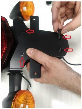
18) Route the turn signal wires to the top of the assembly through the hole and into the wire channel, use the cable tie to secure the wires in place
