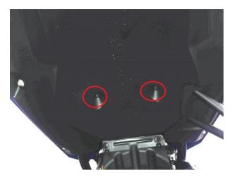
4) Remove the 4 silver 10mm head screws from the undertail assembly and the steel stiffener piece
