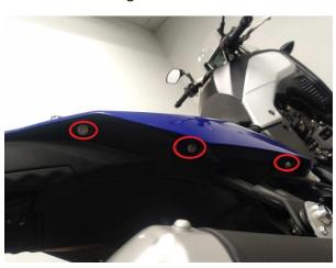
3) Remove the 2 black 8mm head ¼ turn fasteners from the undertail assembly
