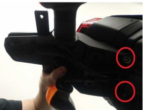
23) Install the 4 silver 10mm head screws and metal stiffener piece to the underside of the tail
