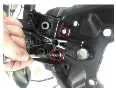
21) Install the taillight/bracket assembly onto the motorcycle, route the harness toward the connector, engage mounting tab into slot on the plastic tail cover
