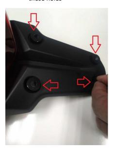
17) Place the Graves Feder Eliminator bracket on to the stepped spacers, Install the 2 flat head and 2 dome head screws, washers, and locknuts to fasten the Graves FE bracket to the OE fender
