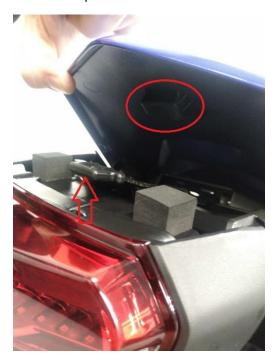
22) Install the Fender Assembly onto the motorcycle using the two silver 8mm head screws, take care to route the wires correctly
