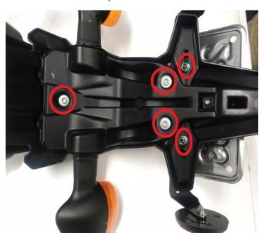
13) Remove 4 silver 8mm head screws from the top of the OEM fender assembly
