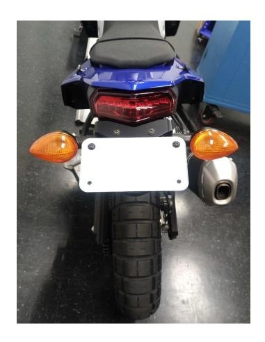
Remove rear seat assembly to access and remove the 5 black button head screws with a 4mm allen wrench
