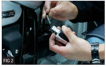
**NOTE:** Install the right passenger foot peg on the left bracket #A00834 and the left passenger foot peg on the right bracket #A00833.
