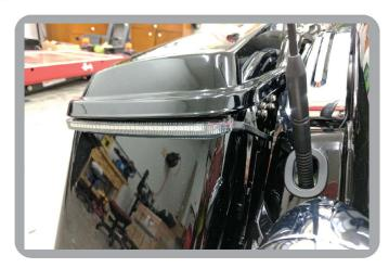
5. Remove adhesive backing from tape and install Bag Blade onto saddlebag, one side at a time. Press and hold firmly for 60 seconds. Adhesive fully cures within 24 hours.
