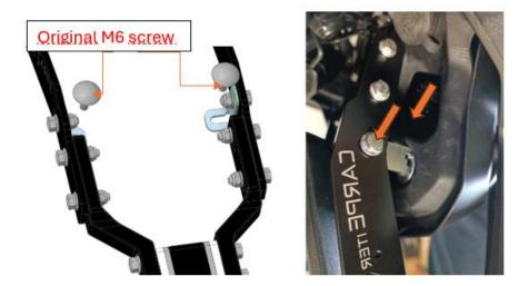
11. Align the bracket parts highlighted in the graphics (orange faces) and tighten screws marked by the yellow arrows (do not tighten the screws for cockpit reinforcement, yet). Recommended toque for M6 screws: 8Nm. Recommended toque for M8 screws: 15Nm.
