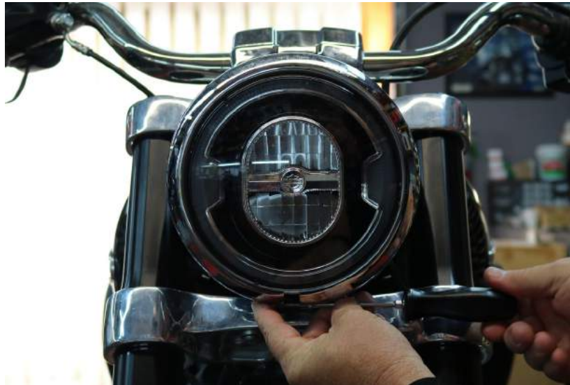
1. Removing Outer Trim Ring
