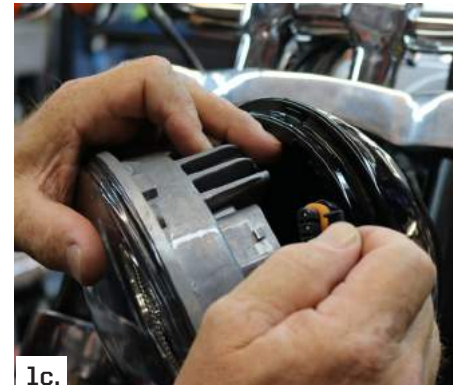
1c. Remove Harness From Headlight
