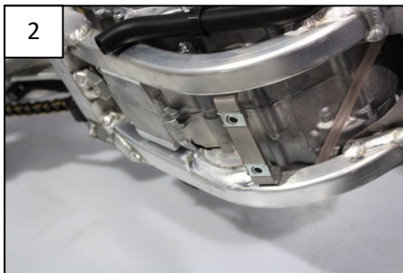
2 Put the front bracket in place Mettre la bride en place
