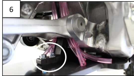
PM01-04-161 + TFHC 6x25mm + washers + em6f Put the rear plastic mount in place Mettre le contre crochet en place
